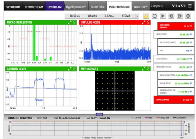
Figure 11. VSE-1100 Packet Dashboard display with impulse noise causing code Word errors
