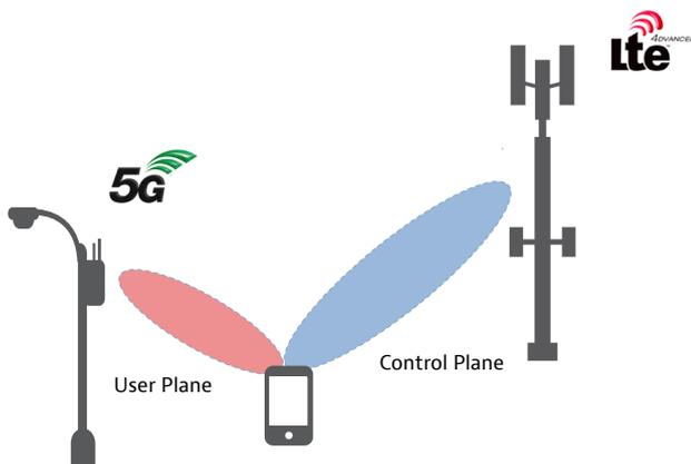
5G NSA allows mobile devices to establish a connection with a master LTE node (anchor) for control plane services, as well as the connectivity to a secondary 5G node for user plane service such as downlink data.
