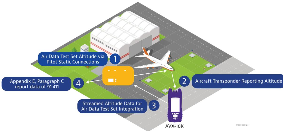
Now, when the Air Data Test Set program is stepping through the various altitudes, instead of asking the user for verification of the transponder reported altitude (Mode C responses), the streamed data from the AVX-10K can be used. Talk to the provider of your Air Data Test Set to find out if they have integrated this new VIAVI feature into their test application!
