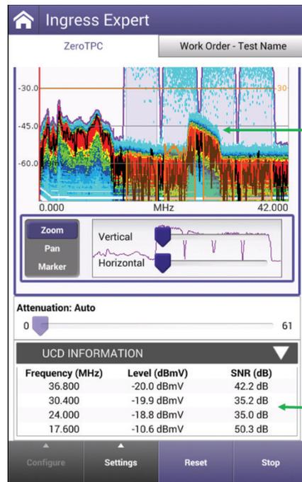
The impact of the noise floor can be clearly seen in the SNR calculated for the 24 and 30.4MHz carriers
