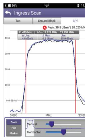
The Ingress Expert FFT display shows a more complete representation of the actual noise signature at any given moment, and with its “Live Max” mode the captured signal remains on the display longer, making it easier for the troubleshooting tech to notice its presence, and perhaps to identify by signature the likely source (in the case above, the characteristic “haystack” of an HPNA signal).
