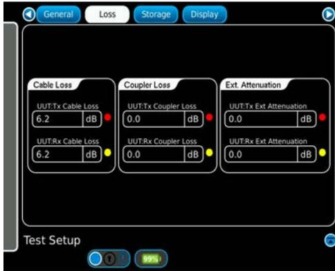
Fig. 15 Test Setup / Loss Tab Screen
