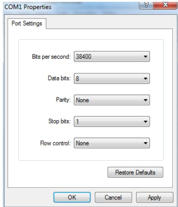
3. Connect to the 860 DSPh by selecting **OK** and then press **ENTER**. The 860 DSPh prompt will be displayed as follows;
