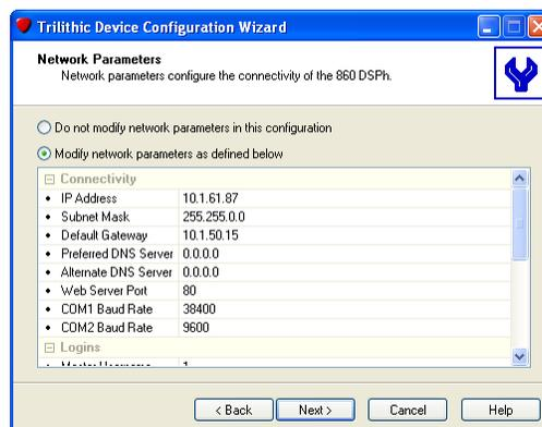
**Alternate DNS Server:** Enter the alternate DNS server's IP address. (This field is required if trap destinations are set as text instead of IP addressed.)
