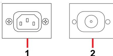
1. **100-240 VAC (US Units)** - AC Power Connector using 110-240 VAC 1A line voltage. This option includes a built-in transformer which is set to the specified line voltage at the factory.
