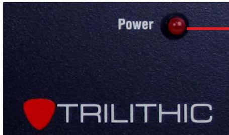
**Power Indicator LED (Red)** - This LED be ON when the 860 DSPh Input Expander is connected to a powered 860 DSPh using the included control cable.
