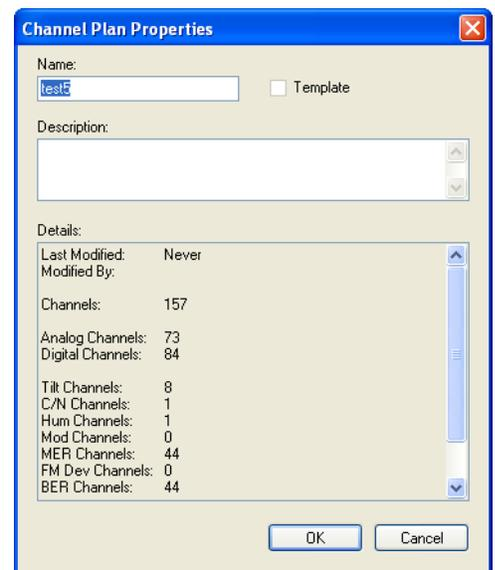
**C/N Channels:** Displays the total number of C/N test channels in the channel plan.
