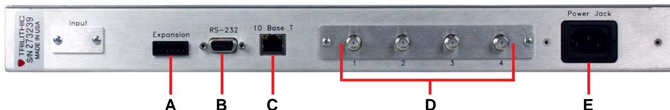
A. **Expansion** - Control cable connection for optional 860 DSPH Input Expander
