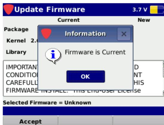
4. If the firmware installed in the 802 AWE is not current, select the **Download** softkey as shown in the image to the right to download the firmware file.
