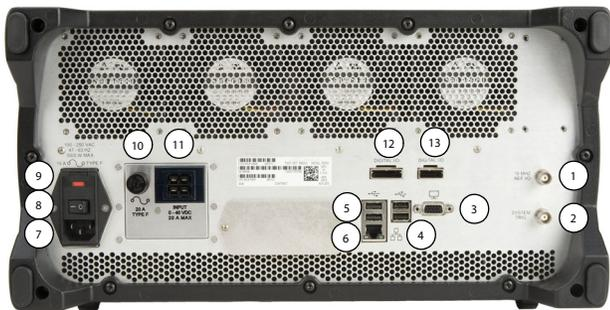
Fig. 2 Test Set Rear Panel Controls/Connectors
