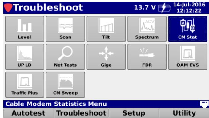
The **Cable Modem Statistics** screen provides the ability to display up to eight (8) downstream or four (4) upstream DOCSIS cable modem channels.
