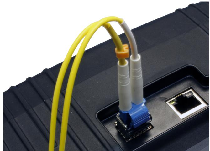
3. Connect the other end of the patch cable to the desired test point within the network (e.g. network switch or router). Once the patch cable has been attached to the network device, the **Gige Testing** screen will display the link status and speed as shown in the images below.
